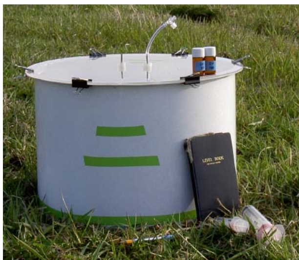
Figure 2.5 Measurement conditions for CH 4 and N 2 O uptake and emission by a chamber method (Shizunai observation site).
