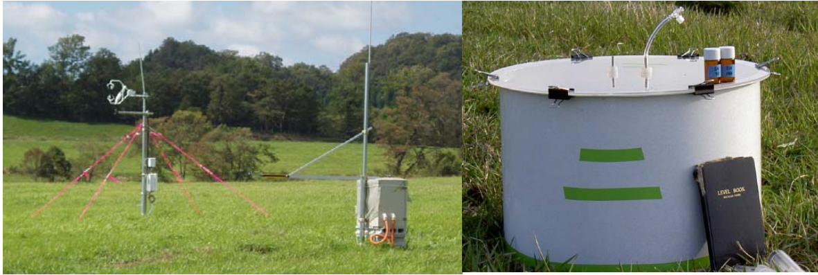
Photograph. Measuring CO 2 by an eddy-covariance method (left) and CH 4 and N 2 O by a chamber method (right)
