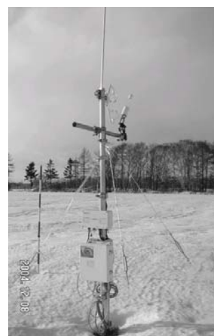
Figure 3.2.2 Measurement device for eddy-covariance method
